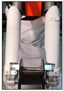
43. Install the ski onto the spindle: Make sure that the thick side of the ski rubber is toward the front. Adjust the bike so that the spindle bottom is slightly higher than the ski. Place the ski under the spindle and lift up on the front of the ski to pull it up into place. Note: it will be a tight fit between the ears of the ski bracket. Push the bolt through and install a lock washer on each side of the bolt. Torque the nut to 50 ft.-lbs.
