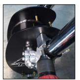
42. Reinstalling the fork guards: It is optional to reinstall the fork guards. To do this you will need to modify them to fit around the fork clamps. First hold the fork guard up into place and free hand draw a line where they will need to be cut. Use tin snips to cut out this portion of the fork guards. Install them on the bike using only the two outside screws. The inside screws will not be used due to the portion being cut away.
