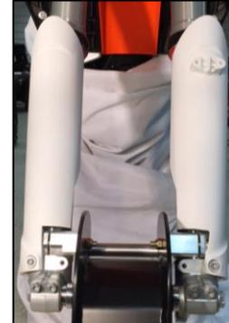
50. **Install the ski onto the spindle:** First make sure that the thick side of the ski rubber is toward the front. Adjust the bike so that the spindle bottom is slightly higher than the ski. Place the ski under the spindle and lift up on the front of the ski to pull it up into place. **Note:** It will be a tight fit between the ears of the ski bracket. Push the bolt through and install a lock washer on each side of the bolt. Torque the nut to 50 ft.-lbs.
