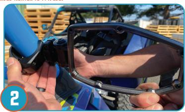
With open side facing forward (allows for windshield), Position the mirrors in desired location on A-Pillar of cage and tighten.
