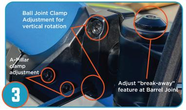
Loosen ball joint clamp, adjust vertical rotation as shown. Once desired position is acheived, tighten all Bolts to secure, then adjust the tightness of the break-away feature and repeat for opposite side mirror.
