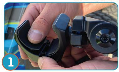
Remove mirrors from packaging and place the rubber clamp bushing appropriate for your cage tube size in the clamp.
