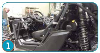
Once Cage has been removed you will need to mask off the area around the plates with masking tape or painters tape and spray paint them so they don't rust.
