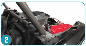
Once the paint dries remove the tape and place the cab section of your new Pro Armor Striker cage into position on the mounting plates.
