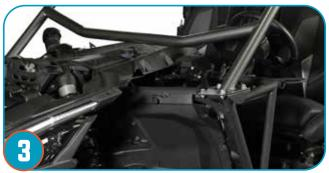
Use 16 m10 bolts and nuts supplied in the hardware pack and fasten cage to mounting plates at each pillar location (4). (washers not needed because both bolts & nuts are flanged!)
