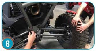
You can now attach the lower part of the rear section to the car using the factory hardware. You will need to wiggle and adjust both rear wheels to align the bolts properly. Don't get frustrated this takes some patience! It helps to raise and lower the car with a jack until you get them aligned. You will not be able to get them all aligned at once so fasten the nuts one at a time until all 6 are on and lined up properly.
