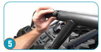
Now you are ready to install the rear section of the cage. You must install it to the cab section from the top first. Fasten with the 4 M8 Allen head bolts into both bungs.
