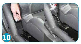
Place the other 2 spacers on the stud and re-use the 2 nuts that were removed in step #4 in the seat base installation. Tighten the 2 nuts with a 18mm socket.
