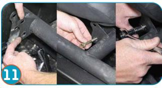
Now align the front of the seat sliders in the bracket and re-use the 2 bolts that were removed in step #3 of the seat base install instructions. Tighten with a 13mm wrench and socket.
