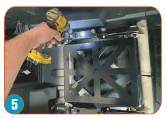
With both seat sliders removed from the car place your new pro armor seat base on and align with the 4 bolts. Re-use the stock bolts that were removed in step 1. Use a 13mm socket.
