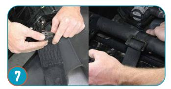
At this point you will either install the stock seat belt to the side of the seat slider or new Pro Armor harness. (harness is recommended)
