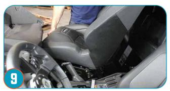
Place the seat in the car and drop the sliders on to the studs so that they are resting on top of the spacers.
