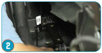
Remove the lower bolt for the stock seat belt with a 16mm socket or wrench. \*Skip step 3 & 4 when installing rear seats.
