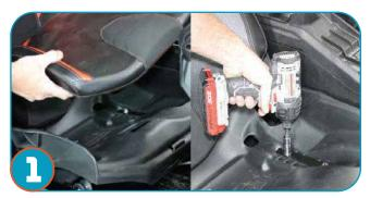
Remove the cushion from the stock seat. Using a 13mm socket, remove the 4 bolts.
