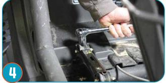
Then remove the 2 nuts from the back of the seat sliders with an 18mm socket.
