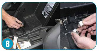
Now you are ready to put the seat back in the car. Place the aluminum spacers on the stud that the seat sliders will be installed.
