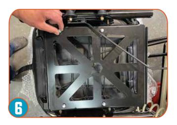
Place your Pro Armor seat face down and attach the seat base to the seat with the 4  $\frac{1}{4}$ -20 bolts that are provided in your hardware pack. Use a 13mm socket or wrench to do this.
