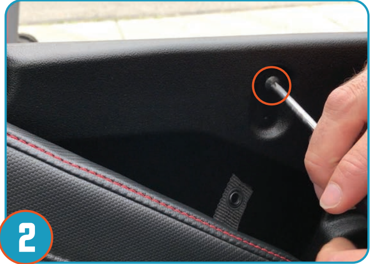
2 Remove factory bolt on stock door, lining up with the front mounting point of the door bag.
