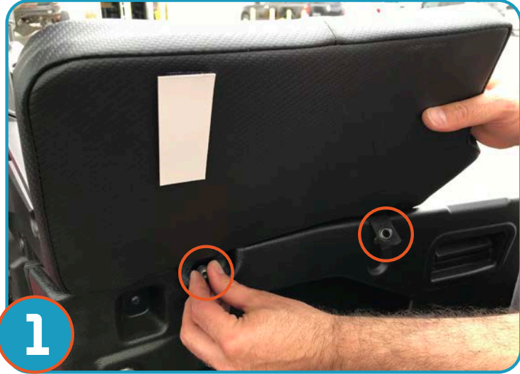
1 Remove bolts from door panel then re-apply and tighten rear portion of door bag while holding in place as shown.
