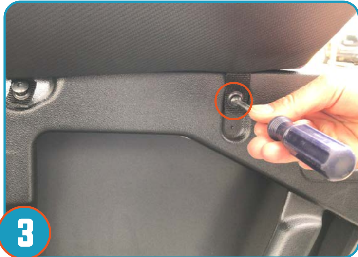
3 Using the same bolt removed in step 2, thread and tighten front portion of door bag.
