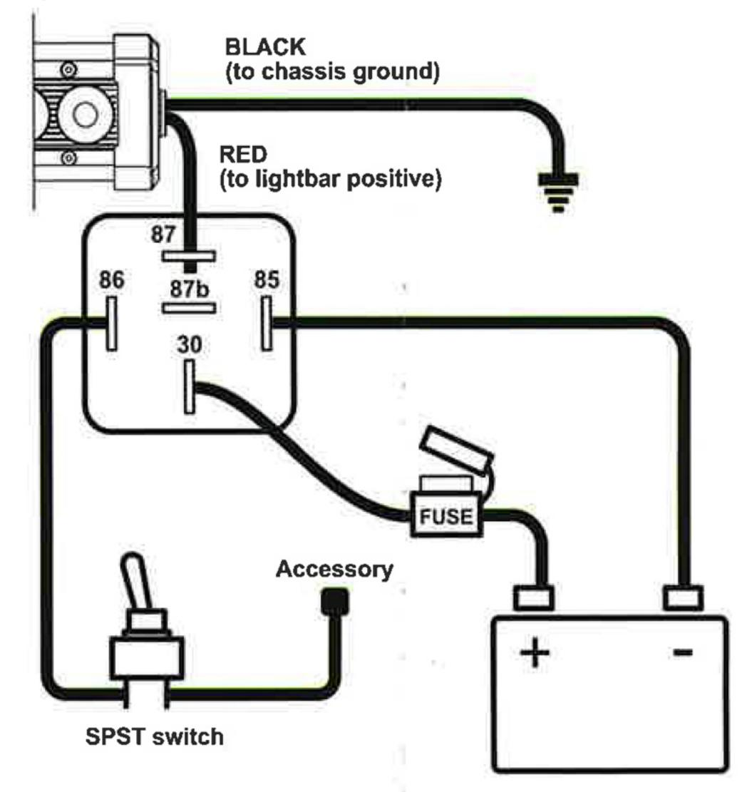
The wiring and connections should be secure and away from any moving parts or extremely hot surfaces
