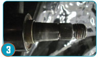
Fully remove the OEM steering wheel and replace it with the steering wheel hub adapter. The hubs fits several models so shaft might differ slightly from picture above.
