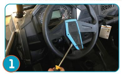
Start the Installation by removing the steering wheel center cap using a flat head screw driver.
