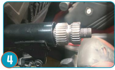
Place the adapter on the steering wheel shaft with the thicker side first. Make sure the tires are straight and the notch on the adapter is top dead center.
