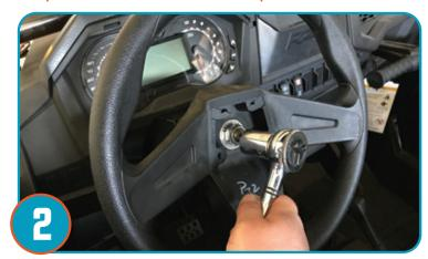
Then remove the center nut with a 24mm socket. Most vehicles require a steering wheel puller to safely remove the steering wheel.
