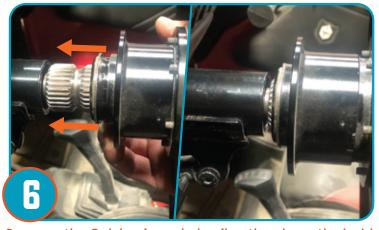
Squeeze the Quick release hub, align the pin on the inside of the hub to the notch on the adapter and install onto the adapter.
