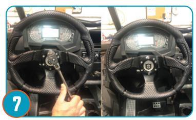
Place the wheel in the right location and tighten the hardware from your wheel down to the wheel manufacturer's specifications.
