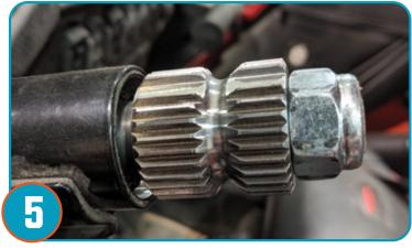
Thread the nut onto the steering wheel shaft, tighten to factory torque specs.
