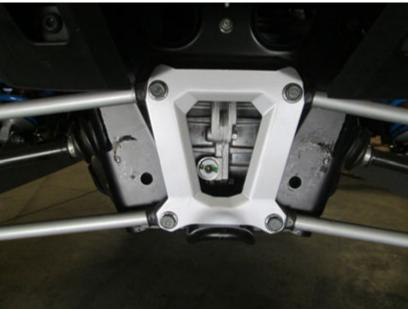
Make sure the lower mounting holes are unobstructed.
