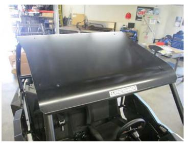
Place roof onto ROPS. Align slots on the roof to the mounting holes on the ROPS. Use the supplied M6 button head bolts, rubber washers, and nyloc flanged nuts to loosely fasten roof [Items 2, 3, and 4].
