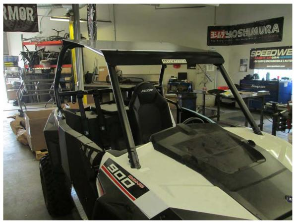
Begin by removing any obstructions that may interfere with the installation of the roof. Place the supplied rubber strips [Item 1] strategically around the ROPS (circled in red), to eliminate any rattling noises.
