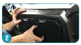
Re-insert the stock grille with the bottom side in first then click the top side tabs into place.
