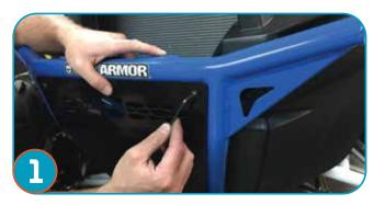
Align skidplate on the front of the bumper and tighten it using the 4 black allen bolts (#1- M6 x 16mm, Button HeadFlange Black Žinc Bolt).
