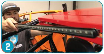
Insert lightbar into rear-wing, running the wire through the back opening of rear wing.
