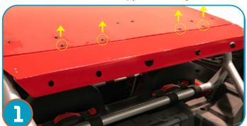
If replacing the rear wing of your Asylum roof with new rear lightbar remove the 4 allen bolts securing wing to roof and replace with lightbar wing replacement and re-apply the 4 allen bolts.
