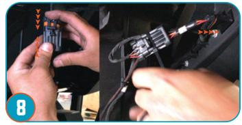
Connect the harness plug to the rear brake plug, then plug into rear brake light port on vehicle. Your rear amber and brake light will now operate with your rear brake lights.
