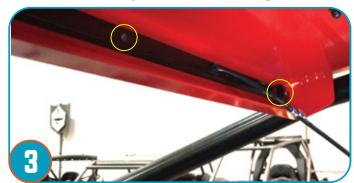
Secure the light-bar to the rear wing using the provided brackets and screws (3 brackets) Using an allen wrench tighten the brackets.
