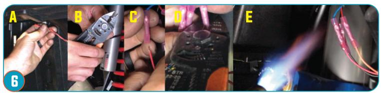
Using the provided wiring harness, connect the light bar wiring to harness wiring. A: Run harness wire to connect to light bar wire. B: Strip wires and join black to black, red to orange, blue to red wires. C: Insert both ends of light bar wire and harness wires into corresponding wire connectors. D: Crimp wires using the provided wire connectors. E: Use torch or heat gun to heat shrink. F: Wrap wire connectors with electrical tape. (not shown above).
