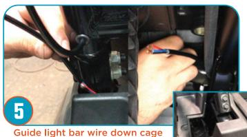
pillar through vehicle plastics into wheel well, running along side the chassis, zip tie as needed to secure wire.
