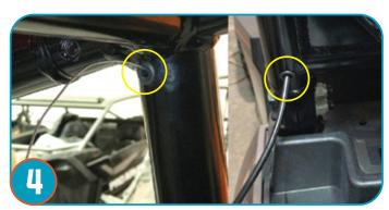
For a clean install, we have drilled holes into the rear cage pillar (Just below weld joint on inside of tube & lower back-side of rear pillar, avoiding welds) and run wires down through tubing. Grommits not included. \*Should you prefer not to drill, your can strategically zip tie the wire.
