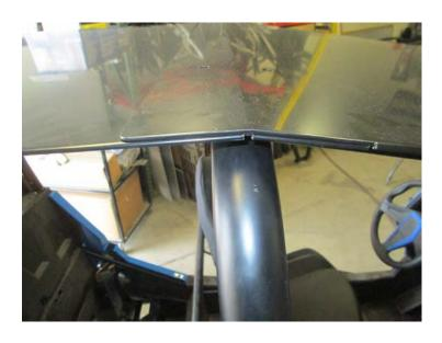
Place the rear half of roof onto ROPS first. Then place the front half, so that it overlaps over the rear half as shown.
