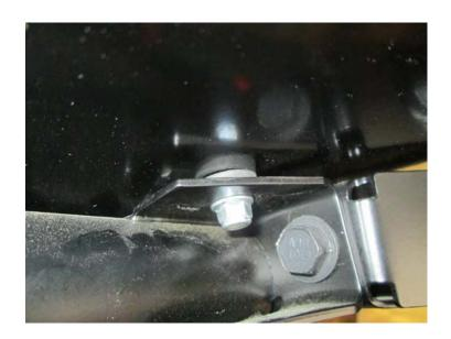
Align the front slots on the front half of the roof to the mounting holes on the ROPS. Use the supplied M6 button head bolts, rubber washers, and nyloc flanged nuts [Items 3, 4, and 5] to loosely fasten the front half of roof.
