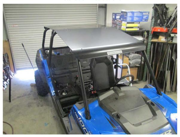
Begin by removing any obstructions that may interfere with the installation of the roof. Place the supplied rubber strips [Item 7] strategically around the ROPS (circled in red), to eliminate any rattling noises.
