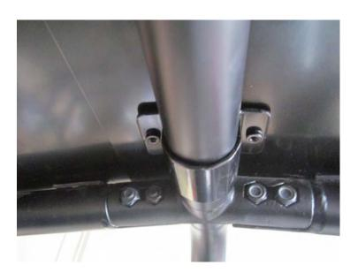
Align the slots on the front and rear halves of the roofs together. Use the supplied middle clamps [Item 1] and the M6 button head bolts [Item 6] to loosely fasten the middle section of the roof assembly.
