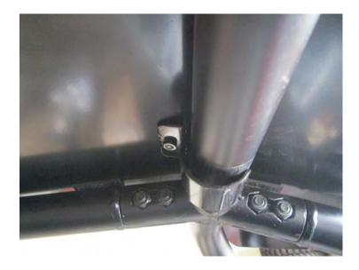
Use the supplied half clamps [Item 2] and the remaining M6 button head bolts [Item 6] to loosely fasten the rear section of the roof assembly.
