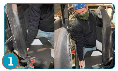
Start the LE rear bench seat installation by first removing the two OEM rear seats. Reach through the space between top/bottom cushions and press the plastic latch to release seat base and remove from vehicle.
