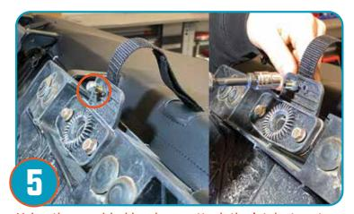
Using the provided hardware attach the latch strap to seat bases as shown for both sides of the bench seat. Tighten nut down to secure.
