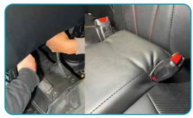
Position the seat base as shown and run the seat belt receivers or Harnesses (depending on whether you have OEM belts or Pro Armor aftermarket harness's) through the slots in bench seat. Click the bench seat in place to secure.
