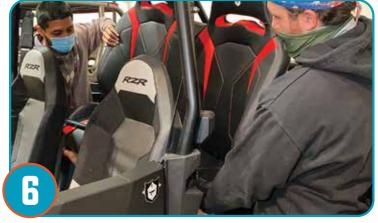
Once the realease straps and bases has been attached and satisfied with placement, the bench can be placed into vehicle.
