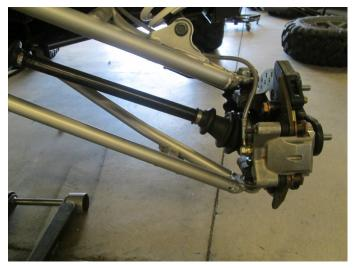
• Place a-arm guard on a-arm and loosely install mounting hardware as shown. Adjust a-arm guard to ensure best fitment. Then, tighten down all hardware.
