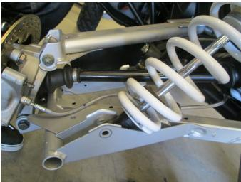
• Place a-arm guard on a-arm and loosely install mounting hardware, including the 15mm lower coilover bolt and nut as shown. Adjust a-arm guard to ensure best fitment. Then, tighten down all hardware.
