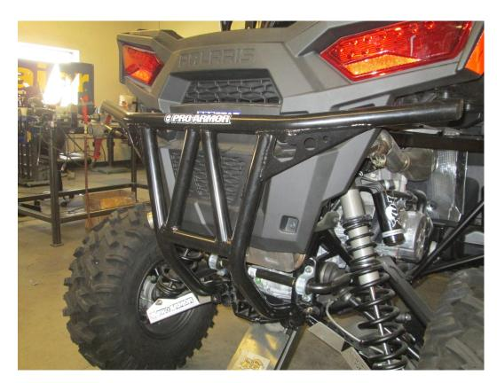
• Replace the 15mm bolt and nut you removed earlier, but without the washer. This will ensure that the threaded portion of the bolt will reach the nylon portion of the nut. It may be helpful to have a second person pull/push on the wheel to realign the mounting holes, while you shoot the bolt through. Leave the hardware loose. Repeat for other side.
