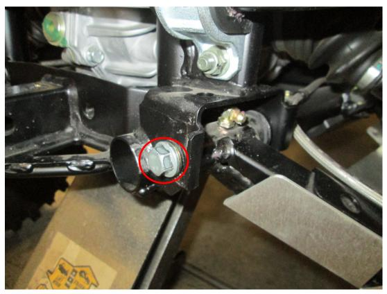
Place the bumper onto the car and line up the lower mounting brackets to the chassis.
