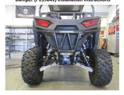
• Begin by making sure there are no obstructions that would interfere with the install of the bumper. Remove the two plastic caps that cover the upper mounting holes.
