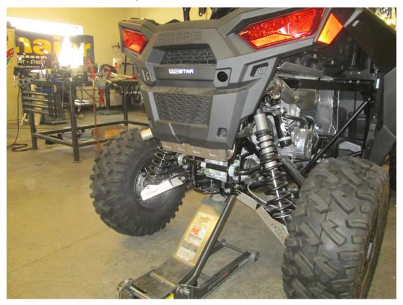
• Remove the 15mm bolt, washer, and nut used to fasten the lower a-arm to the chassis. Repeat for other side.
