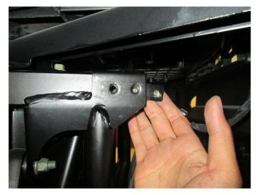
• The supplied mounting tab [Item 2] will be placed on the inside of the chassis' square tube as shown. The supplied M6 button head bolts [Item 1] will then be used to fasten the upper mounting bracket to the chassis. It may be helpful for a second person to hold the mounting tab in place, while you line up the upper mounting bracket and shoot the M6 bolts through. Leave the hardware loose. Repeat for other side.
