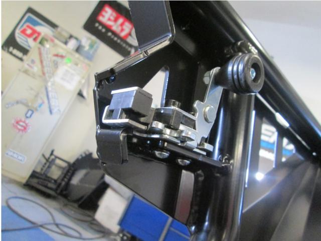
7. Loosely fasten the latch assembly to the door. Use the 30mm M6 button head bolts (Item 10), the latch fastener (Item 3), and the M6 washers (Item 11).
