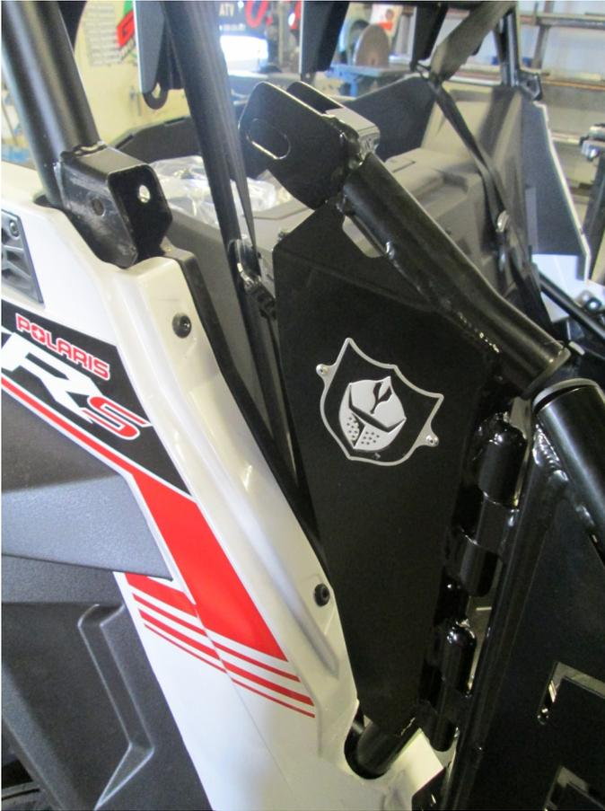
4. Take your Proarmor door and insert the lower mounting bracket through the plastic trim. Then line up the upper mounting bracket to the b-pillar.
