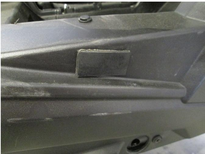
9. Place an adhesive rubber strip (Item 15) where the door meets the plastic trim at the lower front corner. This will eliminate any unwanted audible vibration between the door and plastic trim.
