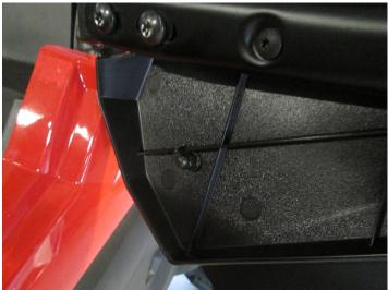
12. Loosely install half clamps to the quarter panel using the provided M6 bolts. Line the quarter panel with the door frame, making sure the edges of the quarter panel run along the center lines of the tube and there is an even gap between the panel and plastic trim. Tighten down hardware.
