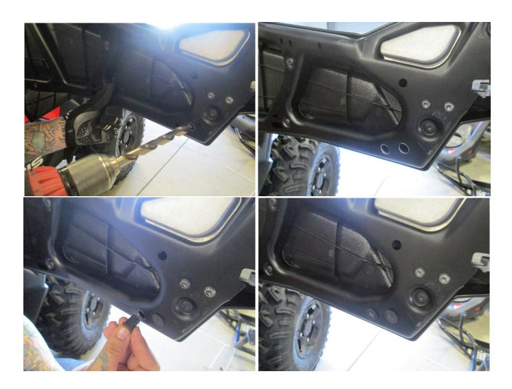
4. Remove the middle, lower T25 Torx bolt. Place door insert on door and line up all mounting holes. Loosely install the 1/4"-20 bolts and washers into the rubber plug-in nuts, as well as the T25 Torx bolt. Adjust door insert to ensure best fit and minimize gaps between door and door insert. Make sure the weather stripping creates a good seal when the door is in the closed position. Fully tighten hardware.
