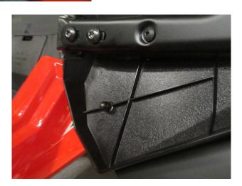
12. Loosely install half clamps to the quarter panel using the provided M6 bolts. Line the quarter panel with the door frame, making sure the edges of the quarter panel run along the center lines of the tube and there is an even gap between the panel and the plastic trim. Tighten down hardware.
