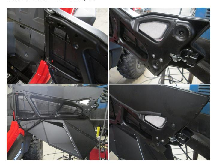
4. Reinstall the upper two T40 torx bolts and hand tighten. Adjust the door along slots to make ensure smooth latch operation. It may be necessary to loosen the lower two T40 torx bolts to do so. Make sure the weather stripping creates a tight seal when the door is in the closed position. Once the door is adjusted properly, torque down any loosened T40 torx bolts. Do not forget to fully tighten the two T25 torx screws as well.
