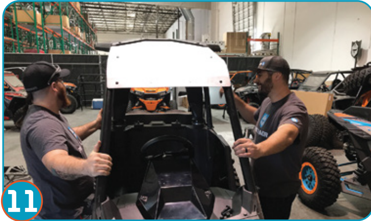
Grab a helping hand, lift and remove stock cage from vehicle.
