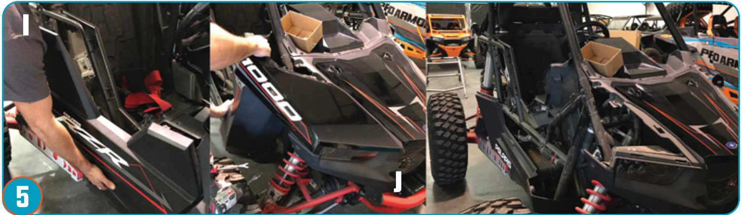
5 (NON-DOOR SIDE) I. Remove side panel plastics. J. Remove front fender plastics. Note: You will need to remove the shocks remote reservoirs, to do this remove the hose clamps that are securing them to the stock cage.
