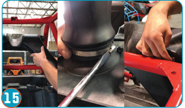
15 Re-apply intake, tightening the adjustable hose clamps removed in step 12 and two bolts from step 9 .
