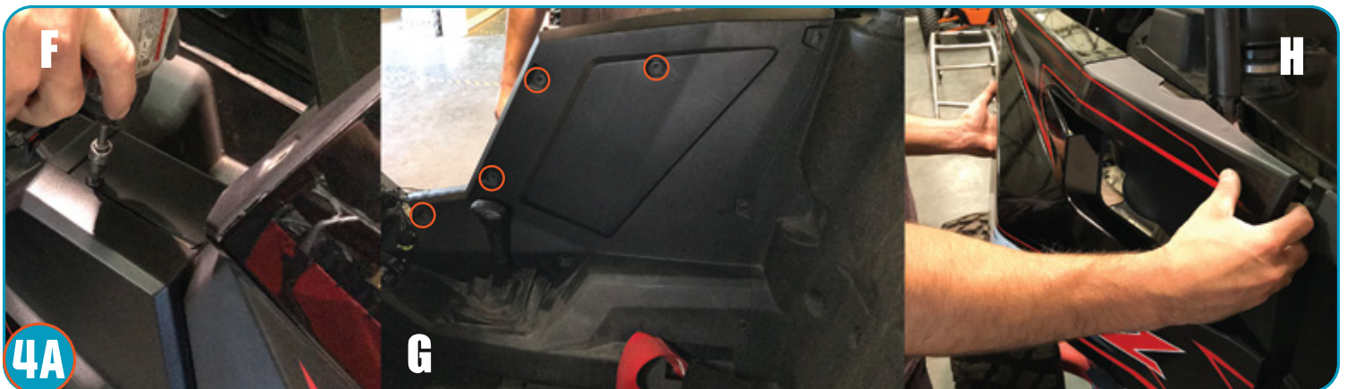
4A (NON-DOOR SIDE) F. Remove top bolt for side plastics. G. Remove four bolts on inside panel. H. Repeat step 3 for rear section of non-door side of vehicle.
