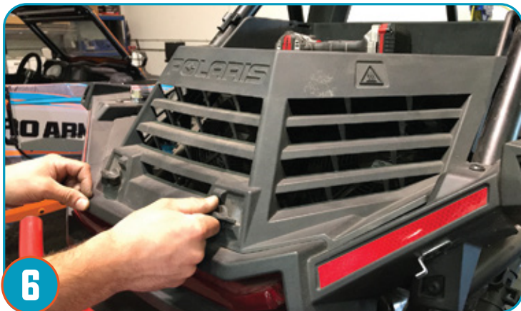
6 Twist (2) quarter turn latches to remove engine vent panel.
