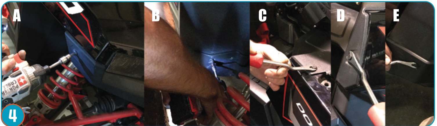
4 (NON-DOOR SIDE) A. Remove bolt Side front plastics. B. Remove two bolts in wheel well. C. Remove push pins top of hood near A-pillar. D. Remove push pin on side of front plastics. E. Remove push pin at bottom of wheel well plastics.
