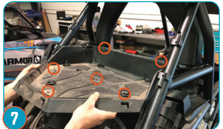
7 Remove 6 bolts to remove rear engine cover plastics.
