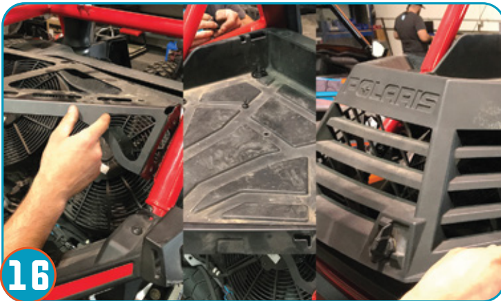
16 Re-apply engine cover bracket (4) bolts & engine cover plastics (6) bolts & engine vent panel, removed in step 6, 7 & 8.
