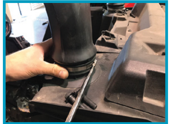
Following the removal of stock cage you will need to loosen the adjustable hose clamps located at both sides and pull upward to separate the intake from the vehicle.
