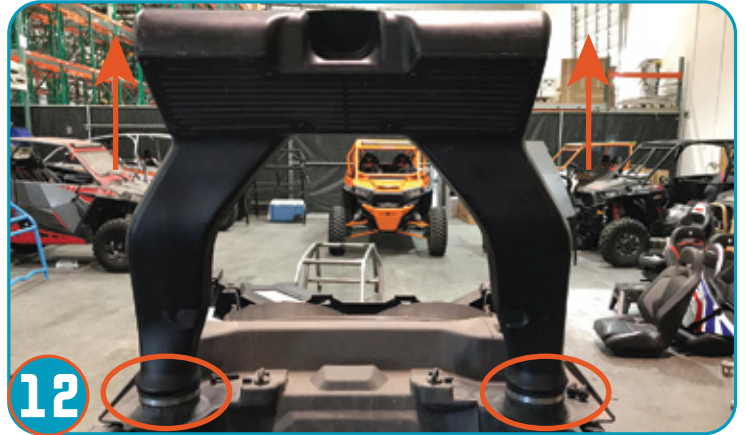
Following the removal of stock cage you will need to loosen the adjustable hose clamps located at both sides and pull upward to separate the intake from the vehicle.
