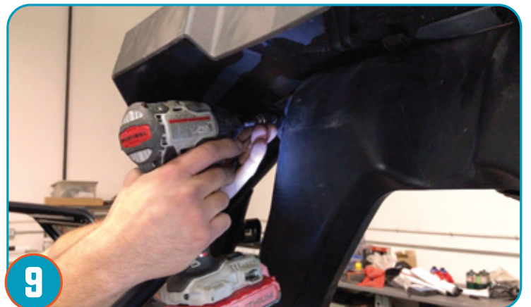
9 Remove 2 bolts to separate Intake from stock cage. 1 bolt per side of intake.
