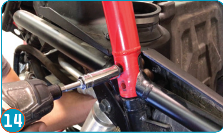
14 Re-apply A,B, C-pillar bolts removed in step 9. Torque to factory specs.
