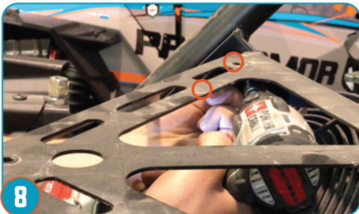
8 Remove 4 bolts to remove rear engine cover bracket, 2 per side of bracket.
