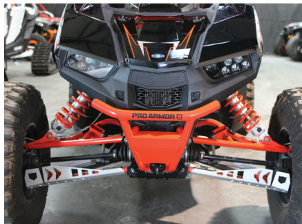
3 Install M10 bolts (2) and factory chasis loop through frame and factory mounting plate then hand tighten.
