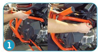
Line bumper up with mouting tabs on rear of vehicle. Hand tighten M10 bolts (2) and nyloc nuts.
