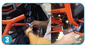
Check to make sure bumper is square on vehicle and properly lined up. Tighten ALL mounting points (upper and lower bolts) to secure bumper.
