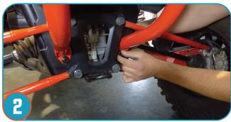
Place lower mounting plates (provided) inside the frame for the lower M10 bolts (2) and hand tighten bolts.
