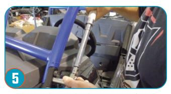
Firmly tighten all hardware to manufacturer's torque specs to secure the cage firmly to the chassis.
