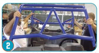
Once the existing roll cage is removed, attach the Pro Armor Cage to the vehicle chassis using the existing hardware at the A and C pillar (Hand tighten). Again, it takes two people to safely handle the cage.
