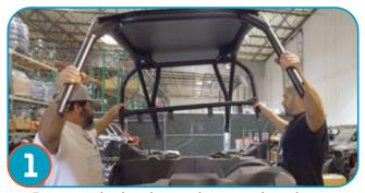
Remove the hardware that attaches the existing roll cage to A-B-C pillars on the chassis of the vehicle. Save all of this hardware, you will need it to attach the new Pro Armor cage. Once all hardware is removed, detach and remove the old cage from the vehicle. It takes two people to safely handle and detach the cage.
