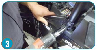
Re-install your doors. Once doors are in place, install B-pillar hardware and check the fit and alignment of the Pro Armor cage.
