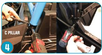
Depending on what doors you have, re-install your doors. Once doors are in place, check the fit and alignment of the Pro Armor cage.
