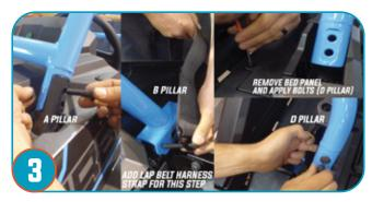
Once new cage is in place, attach the Pro Armor cage to the vehicle chassis using the existing hardware at the A, B, D pillars (Hand tighten). You will want to take this time to install your Pro Armor harnesses lap belts.
