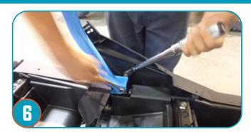
Firmly tighten all hardware to vehicle manufacturer's torque specs to secure the cage firmly to the chassis. Re-install mounting hardware for B-Pillar plastics.
