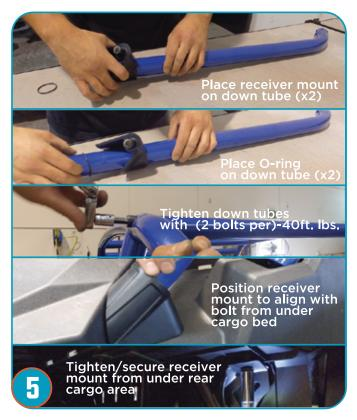
Place provided receiver mount, found in harware kit along with o-ring onto rear down tube bars (x2) to be installed in the rear cargo area. Attach down tubes to cage bungs and align receiver mount. Install supplied bolt and washer at bottom cargo area into receiver mount. (If installing on a Turbo S, use existing stock hardware already on vehicle).
