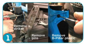
Remove the hardware that attaches the existing roll cage to A-B-C-D pillars on the chassis of the vehicle. Remove B-Pillar plastics as shown. Save all of this hardware, you will need it to attach the new Pro Armor cage.
