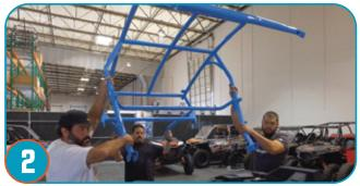
Once all hardware is removed, detach and remove the old cage and place Pro Armor cage on vehicle. It takes two, preferably 3, people to safely handle the cage on and off vehicle.
