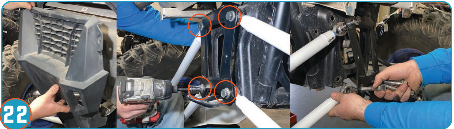
Remove cover providing access to radius rod plate, jack up rear of vehicle and remove 4 bolts securing the rods to the plate. Allow the radius rods to gently fall to floor and discard plate. Plate will no longer be required.
