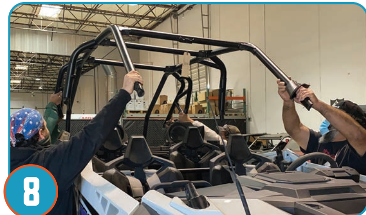
With all the bolts removed from the stock cage and with help from 3 friends, carefully lift and remove stock cage.
