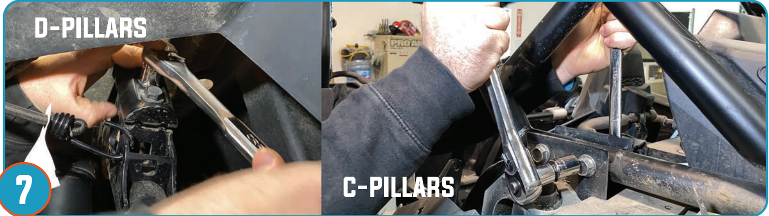
Remove cage bolts starting at the rear D-pillars (4) C-pillars (4).
