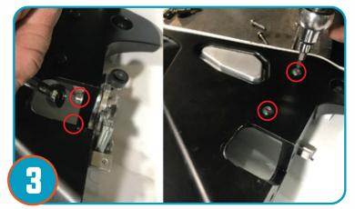
Remove four bolts holding OEM Paddle latch on the stock rear door. Repeat for opposite door.
