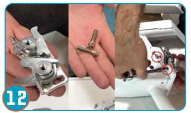
Attach the slam latch to the door using 2 bolts removed from step 3. Only Thread half way. Repeat for opposite door.
