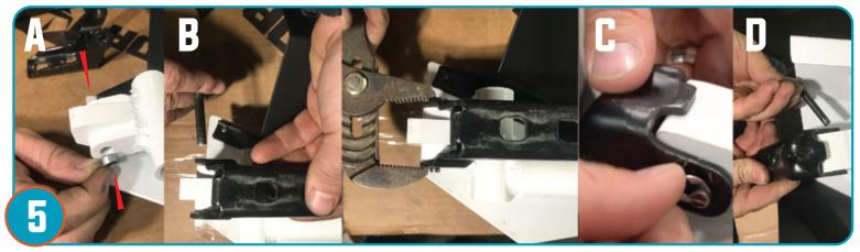
A. Insert bushings removed from step 2 for top and bottom hinges of the Pro Armor door. B. With the inside of the door facing up, place stock hinge as shown in picture. Insert pin through lower hinge. Firmly squeeze door hinge to ensure pin is all the way through. C. Install C-clip on pin. D. Repeat for upper hinges. Repeat for opposite rear door.
