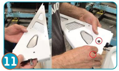
Attach the paddle latch to the latch plate using 2 bolts removed from step 3. Only Thread half way. Repeat for opposite door.
