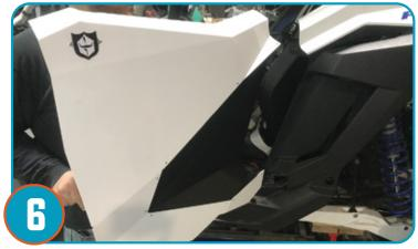
Position door on vehicle lining up hinge bolt holes to door frame hinge. Use provided hardware to hold door in place.
