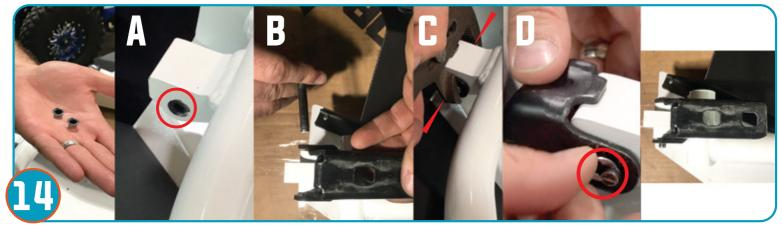
A. Insert bushings removed from step 2 top and bottom of the hinge of the Pro Armor door. B. With the inside of the door facing up, place stock hinge as shown in picture. Insert pin through hinge. C. Install clip on pin. D. Firmly squeeze door hinge to ensure pin is all the way through. Repeat for remaining 3 hinges for both doors.
