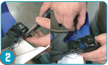
Stock hinges will be used for your Pro Armor door. Remove hinge by carefully removing the C-clip & sliding the pin from the hinge. Remove hinge from stock door. Remove bushings from door. Repeat for opposite door.
