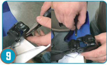
Stock hinges will be used for your Pro Armor door. Remove hinge by carefully removing the clip and sliding the pin from the hinge. Remove hinge from stock door. Remove bushings from door. Repeat for opposite door.
