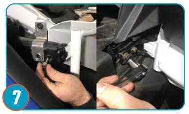
Secure door with bolts provided (2) upper, (2) lower. Adjust door pitch as needed and torque to factory specs. Repeat for opposite door.
