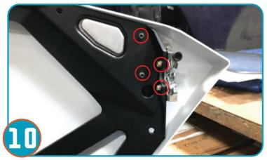
Remove 4 bolts holding the OEM Paddle latch and slam latch on the stock door. Repeat for opposite side.
