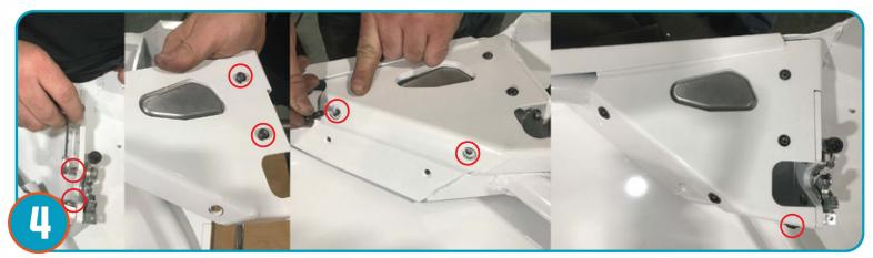
Attach the slam latch & paddle latch to latch plate (provided) as shown with the 4 bolts removed from step 3. Only thread half way. Attach latch plate to door using 4 provided bolts. Secure all 8 bolts.
