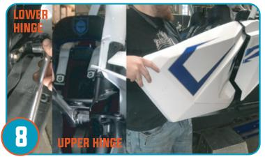
Remove stock door by removing 4 bolts per door and remove lower & upper hinge to remove door from vehicle. Repeat for opposite door.
