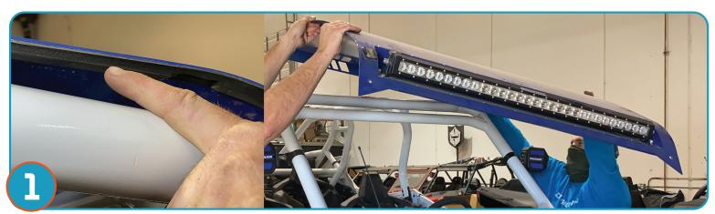
Apply rubber liner along the sides of roof and on cross sections of cage tubing along the middle of cage. With a little help from a friend place roof onto vehicle and line up bolt holes for proper placement.
