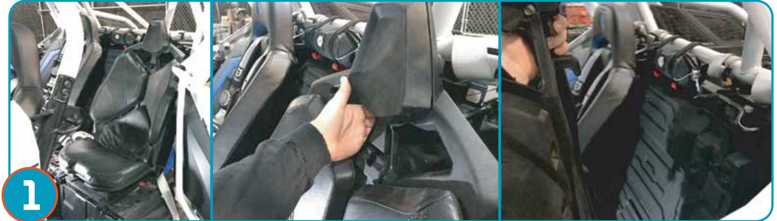
Remove stock seat by lifting the lever located behind the headrest of stock seat. Tilt seat forward to remove.
