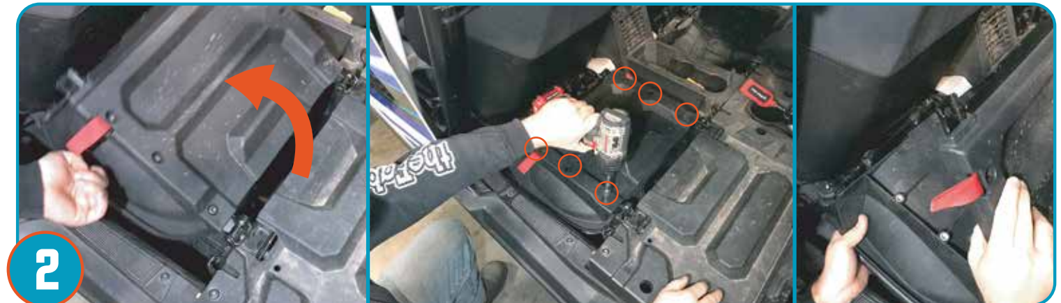
Fold stock seat base forward and remove 6 bolts to remove the stock seat base.
