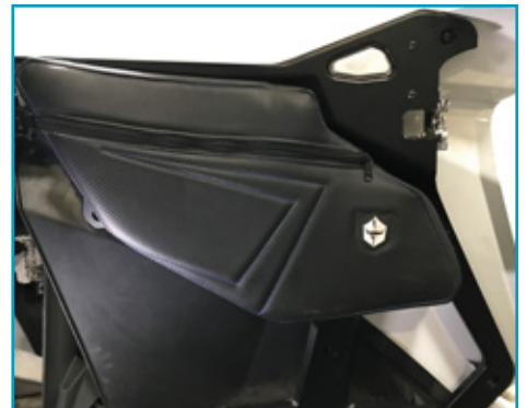
Using the provided three bolts place door bag in place & apply bolts through the zippered compartment aligning inside bolt grommets to the same bolt holes (A,B,C) on door frame that were removed in step 1.
