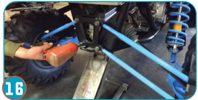
16 Using a car jack, raise rear of car to lift tires slightly off the ground. Remove the radius rod plate to allow arms to move freely.
