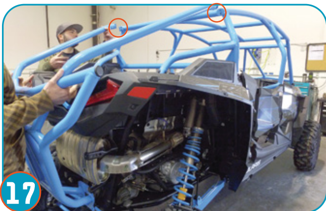
17 Once radius rod plate has been removed let arms fall to allow positioning of rear section. This will be easily accomplished with help from a friend while you insert screws to upper section of cage connecting rear to the main cage while resting radius rod plate on tow hook. Secure top of rear section with provided bolts (2 per side).
