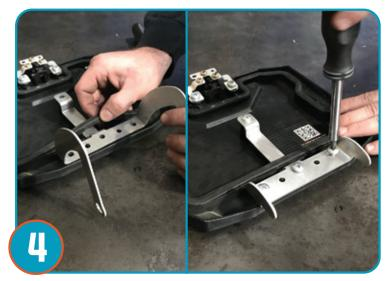
Replace new hinge using the (4) bolts removed in step 1. Slide hinge between rubber gasket and glove box plastics.
