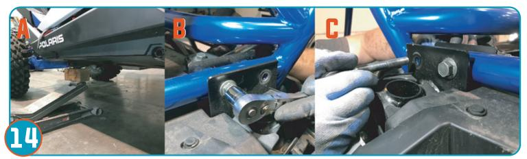
A. Use floor jack to lift vehcile even with B-Pillar location for ease of install. B. Insert B-pillar bolts and torque to factory specs. C. Repeat for opposite B-pillar.
