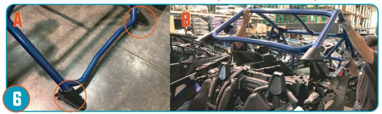
A. Remove A-pillar boots from stock cage and place onto A-pillrs of your new Pro Armor Pro XP cage. B. With some help, lift and place cage onto vehicle, placing rear pillar into place first. Then lower A/B pillars of cage into place.
