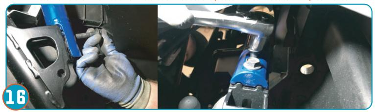
Insert cage bolts removed in step 2D for C-pillar at rear of vehicle. Tighten to factory specs.
