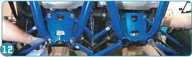
Re-Insert radius plate bolts removed in step 8. Torque to factory cage specs.
