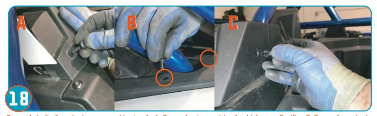
Re-apply bolts & push pins removed in step 1. A. Re-apply at rear side of vehicle near B-pillar. B. Re-apply push pins (2) located on top-side near down tubes as shown. C. Insert push pin on inside B-pillar removed in 1D. Repeat for opposite side of vehicle.
