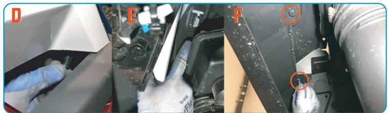
Step 18 (Cont.) D. Insert push pin removed in 1H, at rear plastics above the rear tail light under plastics pushing upward. E. Push plastics clipping in to body plastics (Step 1G). F. Re-apply rear wheel well push pins removed in step 1F. Make sure all bolts and push pins are applied and repeat for opposite side of vehicle.
