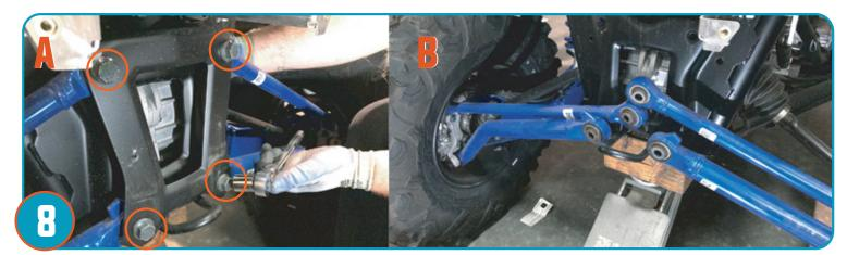
A. Remove (4) bolts to remove rear radius rod bracket. B. Once bolts are removed, remove and set rear plate to the side allowing rear arms to rest as shown.
