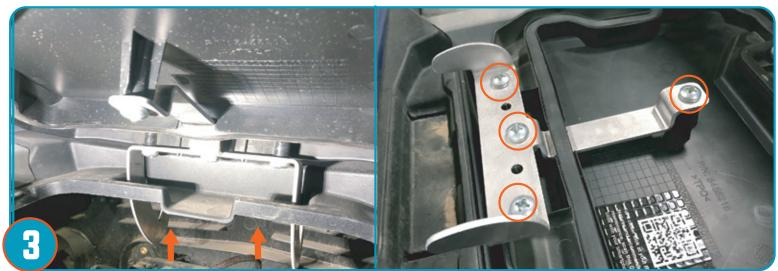
While cage is removed from vehicle, remove glove box and remove (2) bolts at the base of the hinge seperating it from the plastics. Remove (4) screws holding the hinge to glove box panel/lid.
