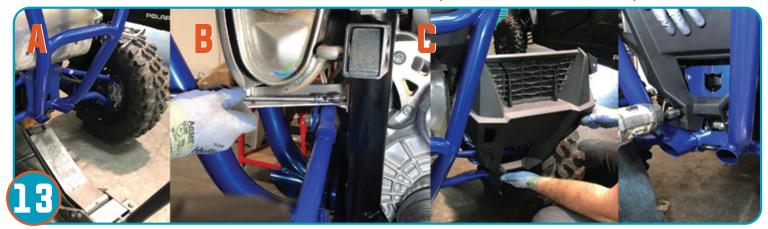
A. Once radius rods and rear section is tightened & secure, lower your jack to original resting position.B. Re-apply brackets (2) using the (2) bolts removed in step 10. C. Re-apply rear exhaust cover plastics using the (4) bolts removed in step 7.
