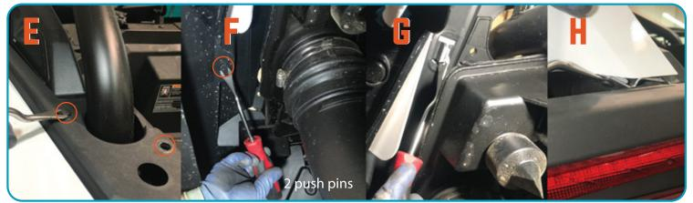
E. Remove push pins (2) located on top-side near down tubes as shown. F. Remove push pins (2) in rear wheel well. G. Depress clip to seperate plastics at top-rear of the wheel well. H. Remove push pin between plastics located between the plastics of the rear tail light assembly.
