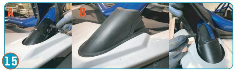
A. Re-apply A-Pillar bolts removed in step 2, tighten to factory specs. B. re-apply A-pillar boot. Repeat for opposite side of cage.
