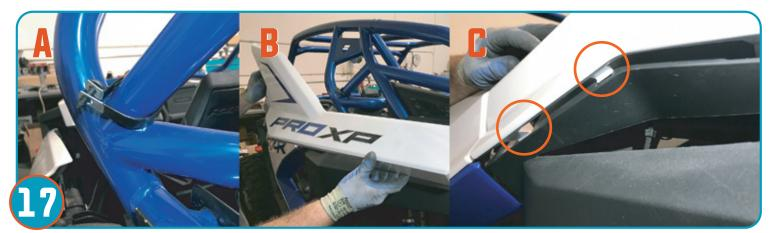
A. Apply plastics bracket in place on cage to be attached to upper arm of plastics and cage in step 19. B. Position vehicle plastics removed in step 11. C. Using clips re-apply plastics to vehicle as shown.
