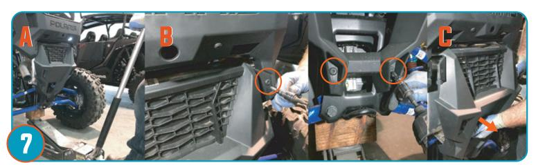
A. For ease of installation jack rear of vehicle up. B. Remove rear exhaust plastics removing (2) upper bolts & (2) lower bolts as shown. C. Remove exhaust cover plastics.
