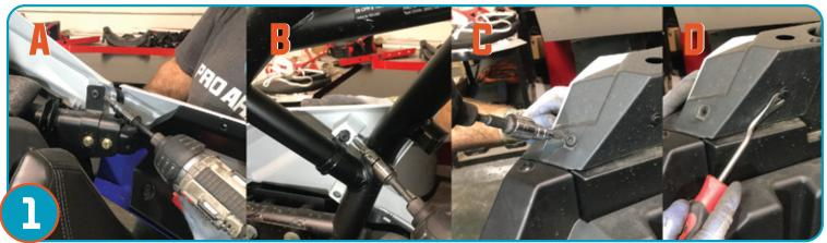
Remove side plastics. A. Remove bolt/bracket at upper hinge as shown. B. Remove B-Pillar bolts located on inside of b-pillar plastics as shown. C. At rear side of vehicle remove bolt as shown. D. Remove push pin as shown.
