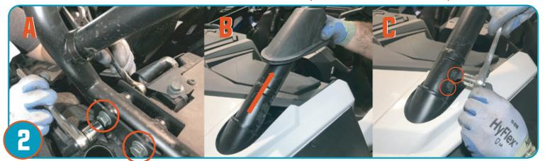
Remove stock cage. A. Starting at the B-pillar, loosen & remove bolts (2). B. Remove A-Pillar boot to expose A-Pillar bolts (2), C. Loosen and remove A-pillar bolts (2). Repeat for oppostie side of cage.
