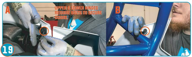
A. Using bolts removed for stock doors in step 1A, re-apply bolts for upper hinge plastics. Adjust doors as needed for proper alignment. Repeat for oppostie vehicle door. B. Tighten the clamp applied in step 17A to secure outer plastics. Repeat for opposite plastics clamp. Installation is complete.
