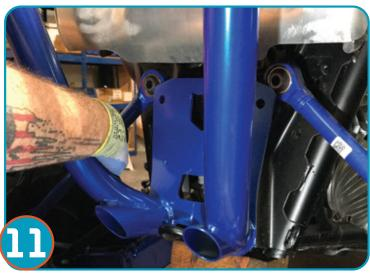
Remove (1) bolt holding two brackets shown for each side Re-position arms in place between vehicle & rear radius rod plate aligning with the bolt holes.
