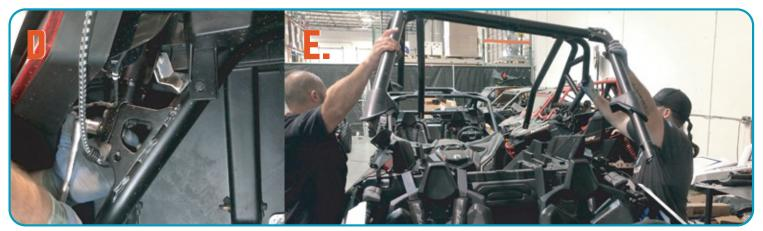
D. Loosen and remove bolts (2) at rear of vehicle and repeat for opposite side. E. With a little help, remove stock cage from vehicle and set aside.
