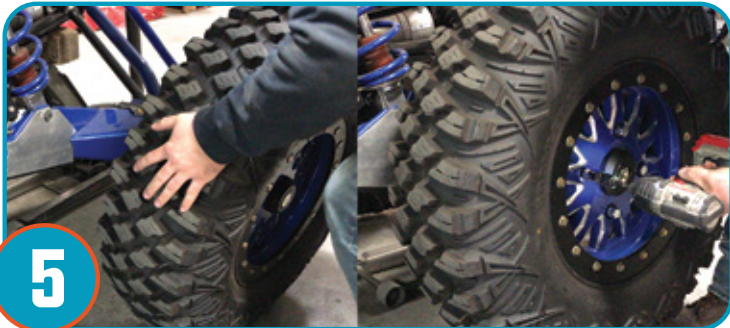
Secure wheel back onto vehicle using a jack, torquing the lug nuts to factory specs. REPEAT FOR OPPOSITE SIDE.
