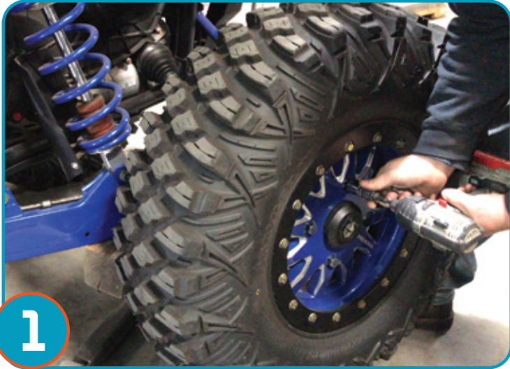
Using a floor jack, raise the rear section of vehicle to easily allow for removal of rear tire. Making sure vehicle is stable, for safety use an additional jack stand.
