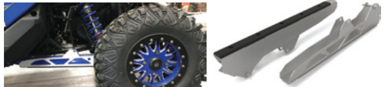
Insert (2) bolts removed in step 2 running the bolts through frame, stabilizing bar link and shock. Tighten securely.
