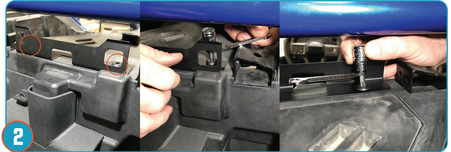
2. Remove OEM brackets by removing two bolts as shown. Repeat for opposite bracket.
