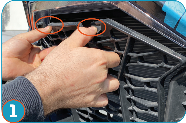
1 REMOVE FRONT OEM GRILLE FROM YOUR VEHICLE, PRESSING DOWN ON TWO TABS.
