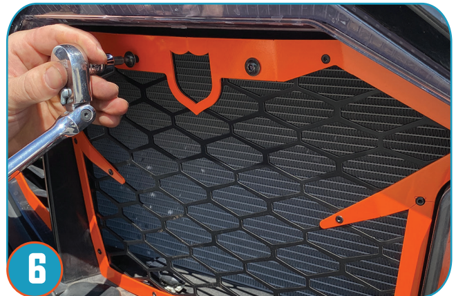
6 SECURE PRO ARMOR GRILLE BY THREADING THE TWO PROVIDED BOLTS (4MM OR H4 ALLEN) AS SHOWN JOINING THE GRILLE AND THE BRACKET INSTALLED IN STEP 5.
