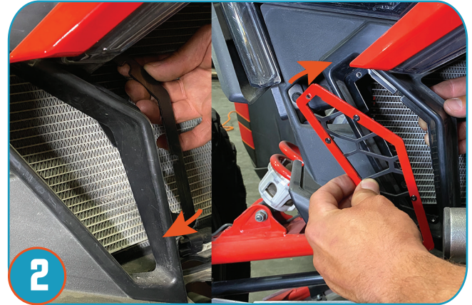
2 START WITH THE SIDE INSERTS, LINING UP THE BLACK BACK-PLATE (PLACED BEHIND PLASTICS) TO YOUR COLOR FRAME (PLACED IN FRONT OF PLASTICS) AS SHOWN.
