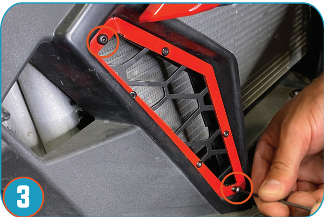
3 THREAD (2- BOLTS) JOINING THE GRILLE FRAME TO THE BACK PLATE, USING A (2MM) ALLEN WRENCH AS SHOWN. +REPEAT FOR OPPOSITE SIDE.
