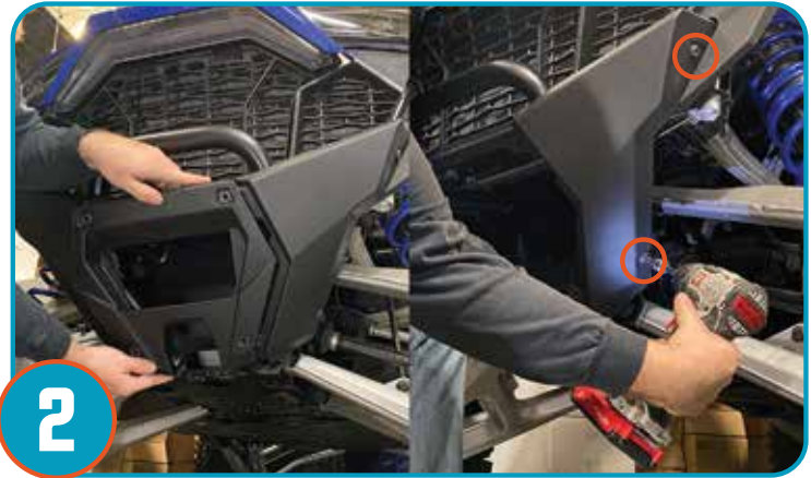
Remove front plate from vehicle and proceed to remove 2 bolts on each side of front bumper plastics, as shown.
