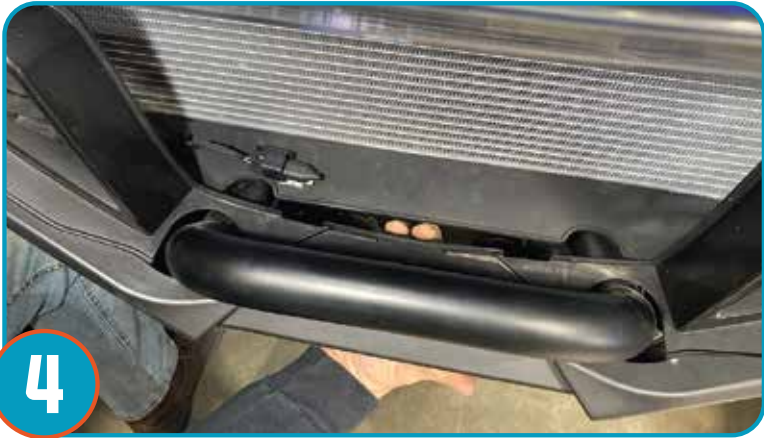
To remove plastics unclip from inside/under front bumper and remove plastics from vehicle.
