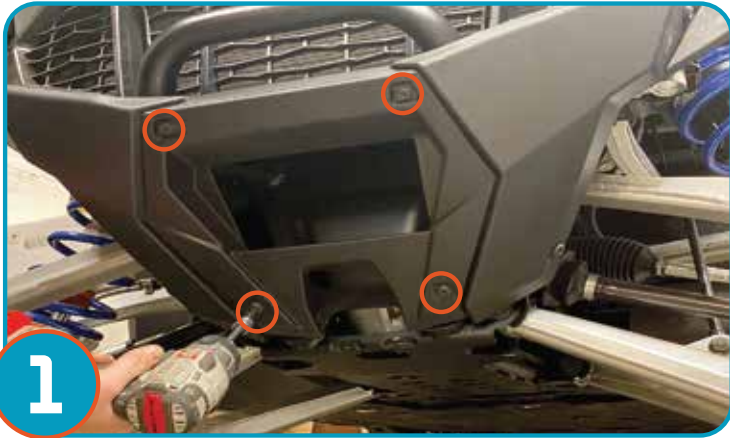
Remove Stock front bumper plate, removing 4 bolts as shown. Stock front bumper plate can be kept or discarded as it will not be returned to vehicle after bumper install.
