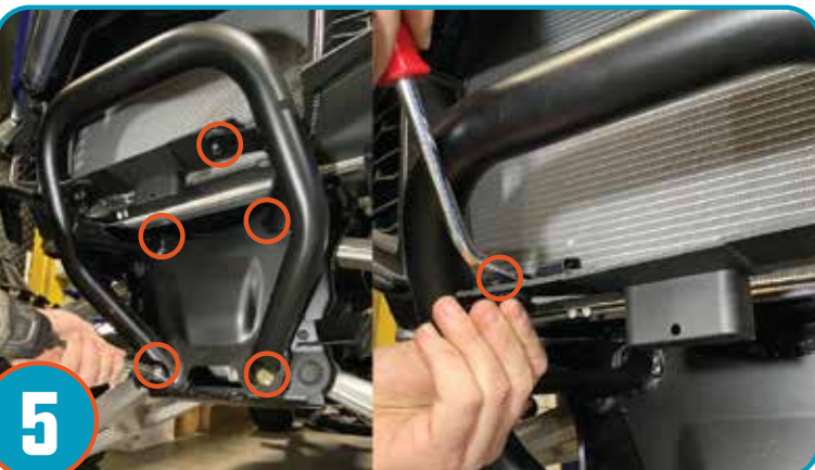
Remove the front 4- bolts & 2 plastic rivet clips as shown.
