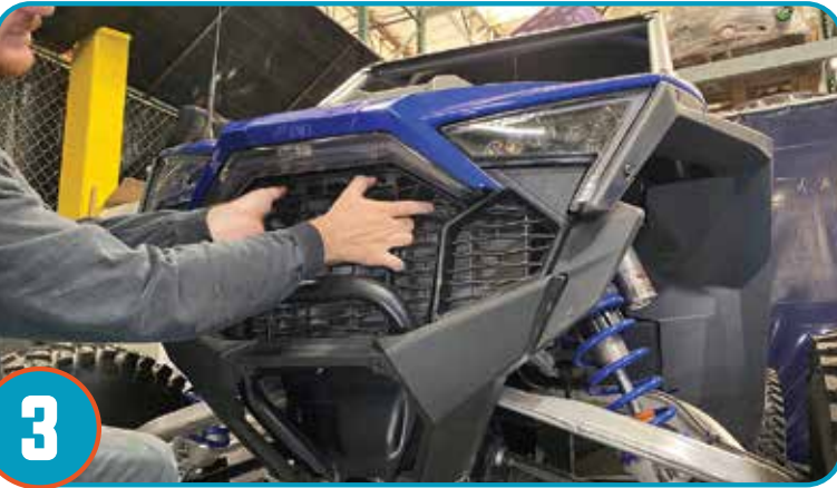
Remove the front grille by depressing the top clips as shown.
