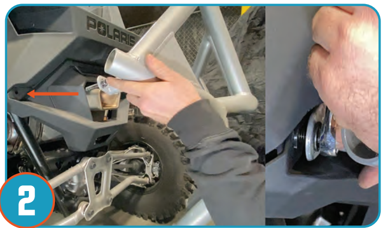
Place your New Pro Armor Rear Bumper aligning upper bolt holes (2), using provided hardware and tighten as shown.
