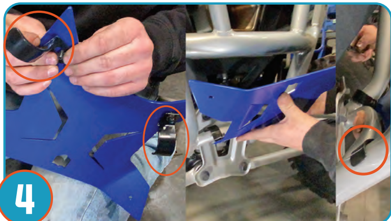
Apply the (2) provided clamps to the bottom rear of the skid plate threading bolts through front of skid, position on bumper lining up bolt holes and position clamps to side tube as shown.
