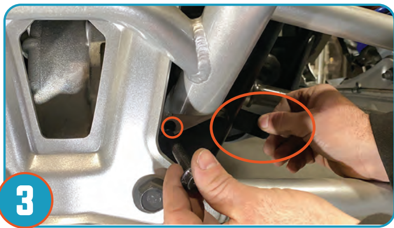
Using the provided back plates thread bolt through lower mounting points while holding the rear plate and tighten to secure rear bumper to chassis.
