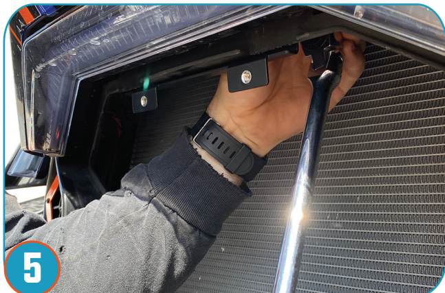
5 USING THE 2-NUTS REMOVED IN STEP 4, PLACE PROVIDED GRILLE BRACKET AND RE-APPLY NUTS TO SECURE BRACKET IN PLACE (DO NOT OVER-TIGHTEN).
