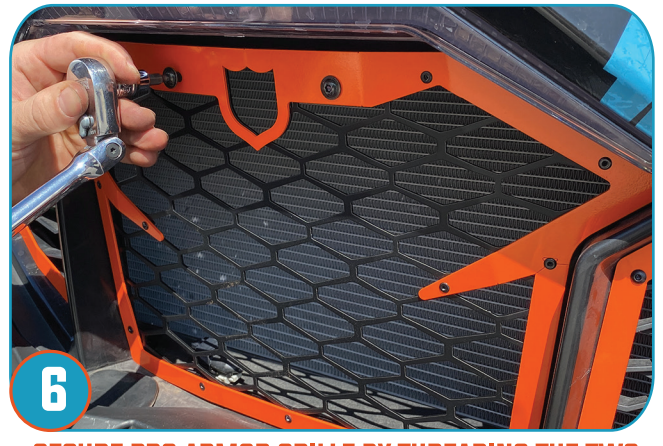
6 SECURE PRO ARMOR GRILLE BY THREADING THE TWO PROVIDED BOLTS (4MM OR H4 ALLEN) AS SHOWN JOINING THE GRILLE AND THE BRACKET INSTALLED IN STEP 5.
