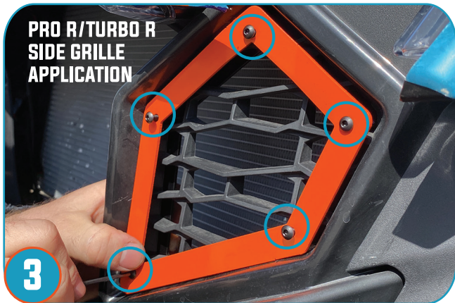
3 THREAD (5- BOLTS) JOINING THE GRILLE FRAME TO THE BACK PLATE, USING A (2MM) ALLEN WRENCH AS SHOWN. +REPEAT FOR OPPOSITE SIDE.
