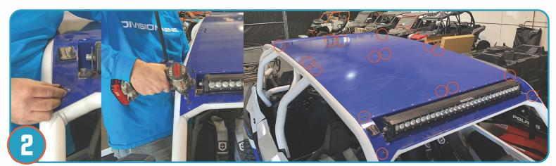
Insert and hand tighten 16 screws then tighten. Do not overtighten.
