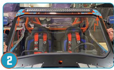
If roof already installed, remove top two roof screws and place windshield on the vehicle, sliding top of windshield under roof and lining up bolt holes. Use provided hardware.
