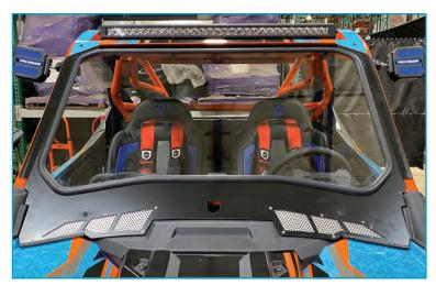
Complete your installation by tightening all four (4) bolt locations to properly secure windhshield to your cage system.
