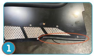
Pre-install prep: Apply provided rubber stripping (if needed) to bottom corners of windshield on both sides as shown. Trim stripping as needed for proper fit.
