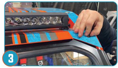
Hand tighten upper windshield with (2) provided bolts threading the bolts into position. One on each of the top corners as shown.
