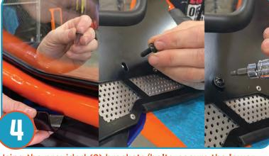
Using the provided (2) brackets/bolts, secure the lower windshield tightening the bracket, threading bolt from outer windshield to cage. One bracket per side of windhshield.
