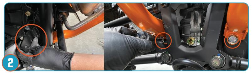
Using the provided back plates thread bolt through lower mounting points while holding the rear plate and tighten to secure rear bumper to chassis.
