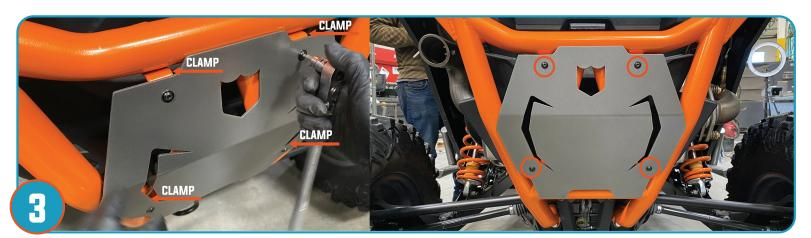
Apply the (4) provided clamps to the bottom and top rear of the skid plate threading 4 bolts through front of skid, position on bumper lining up bolt holes and position clamps on rear tubes to secure rear skid to bumper as shown and tighten bolts (do not overtighten). Install is now complete.
