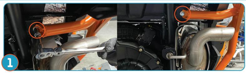
Place your new Pro Armor rear bumper aligning upper bolt holes (2), using provided hardware and tighten as shown for both sides of vehicle.
