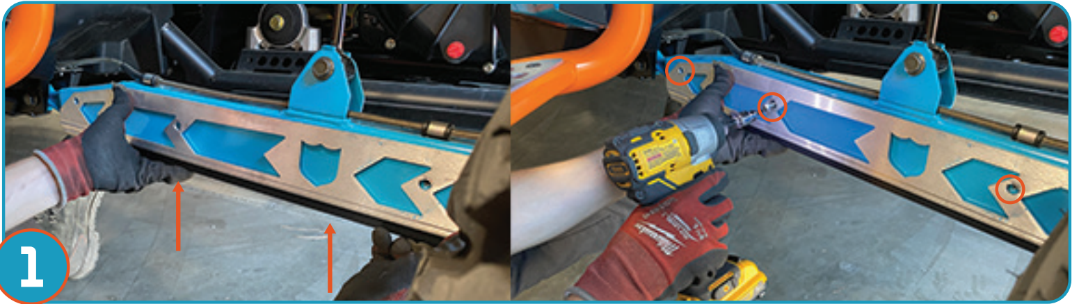
Slide trailing armor up and over trailing arm as shown, lining up (3) mounting holes. Tighten (3) provided, M6 Bolts. Do NOT over-tighten bolts.
