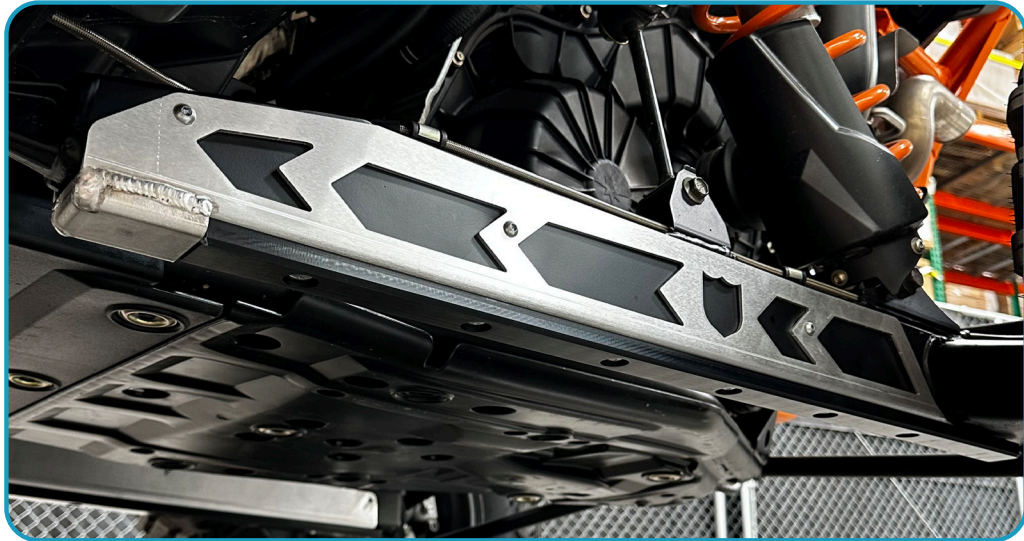
Insert and tighten (3) M6 bolts on the inside of trailing arm and tighten, securing to vehicle. Repeat for opposite side of vehicle. Do NOT over-tighten bolts.
