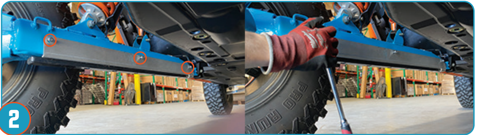
Insert and tighten (3) M6 bolts on the inside of trailing arm and tighten, securing to vehicle. Repeat for opposite side of vehicle. Do NOT over-tighten bolts.
