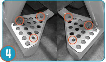
Secure step-plate to rear of rock sliders as shown using provided bolts for both driver & passenger sides.
