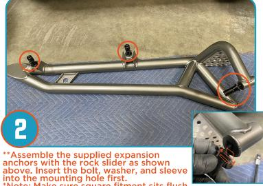
\*Note: Make sure square fitment sits flush to square mounting point as highlighted for rear mounting point.\*\*Refer to anker assembly diagram (Page 2).
