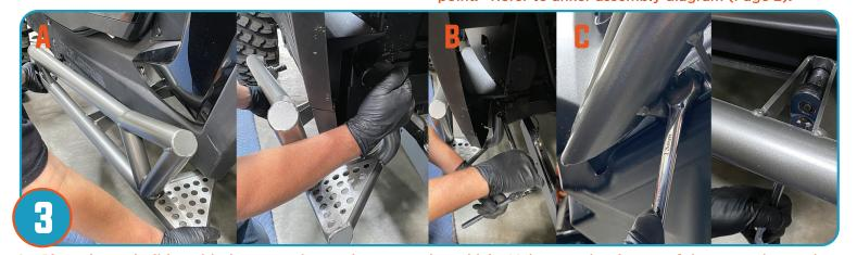
A. Place the rock slider with the expansion anchors onto the vehicle. Make sure the sleeves of the expansion anchors are still seated properly in the grooves in the mounting holes of the rock slider before you proceed to tighten the anchors. Starting at the rear. B. Tighten Rear moounting point. C. Tighten Front & Middle mounting points. Repeat steps for other side.
