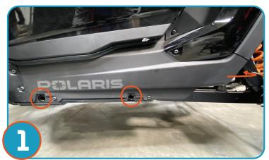
Begin by removing any dirt/obstructions that may interfere with the installation of the rock slider. Make sure all of the mounting holes are clear of debris.
