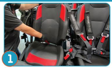
Remove stock seat from vehicle by reaching behind seat and pulling on the release handle (Red)
