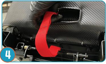
Run the red release strap through rear slot to the front of seat.
