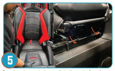
Once base is mounted securely to the seat, place the seat in vehicle angle seat leaning toward the front of vehicle and then back toward the rear of vehicle and click into place. Making sure the seat is properly secure seat.
