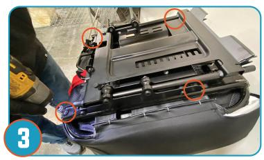
Place the Stock seat base onto your new seat, lining up the mounting holes of base to the new seat. Tighten (4) T27 Torx bolts to secure base to seat. Sliding base for clear bolt access.
