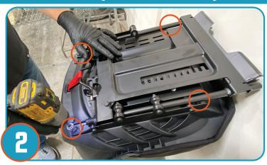
Remove the (4) T27 Torx bolts holding the plastic seat base to the stock seat.
