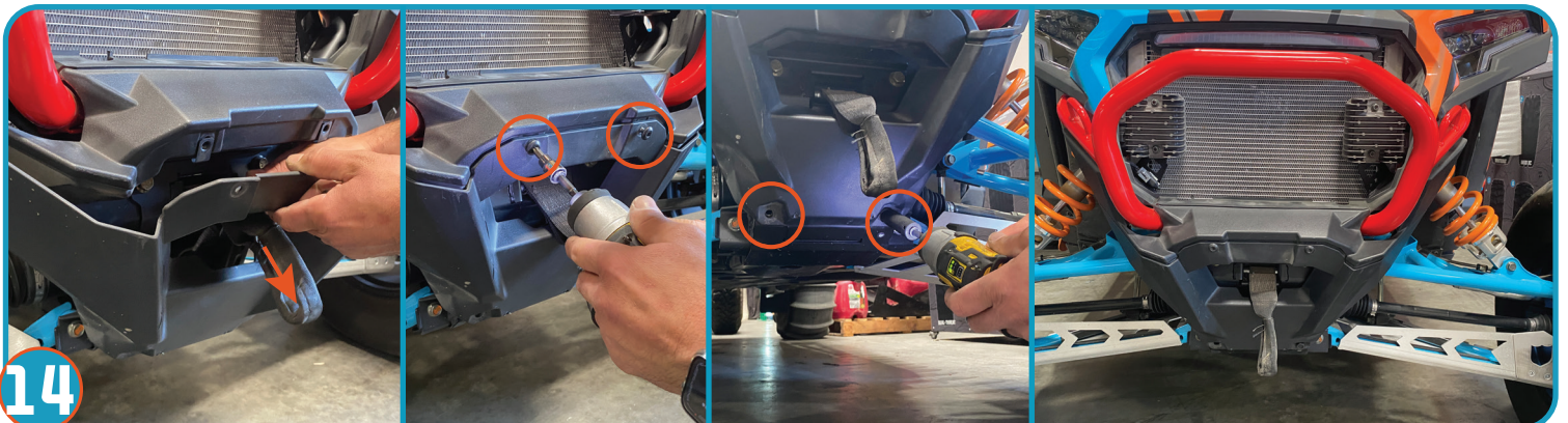
FEED TOW STRAP THROUGH PLASTICS AS SHOWN AND RE-APPLY THE PLASTICS AND BOLTS REMOVED IN STEP 2.
