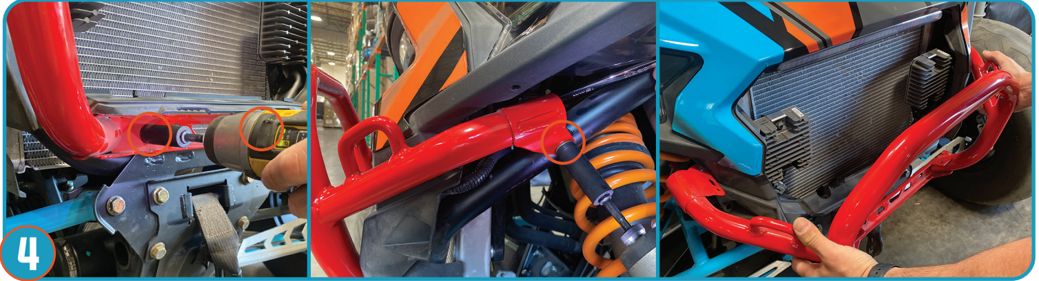
4 REMOVE 4 BOLTS HOLDING STOCK BUMPER. TWO LOWER AND ONE LOCATED ON EACH SIDE OF FRONT BUMPER.
