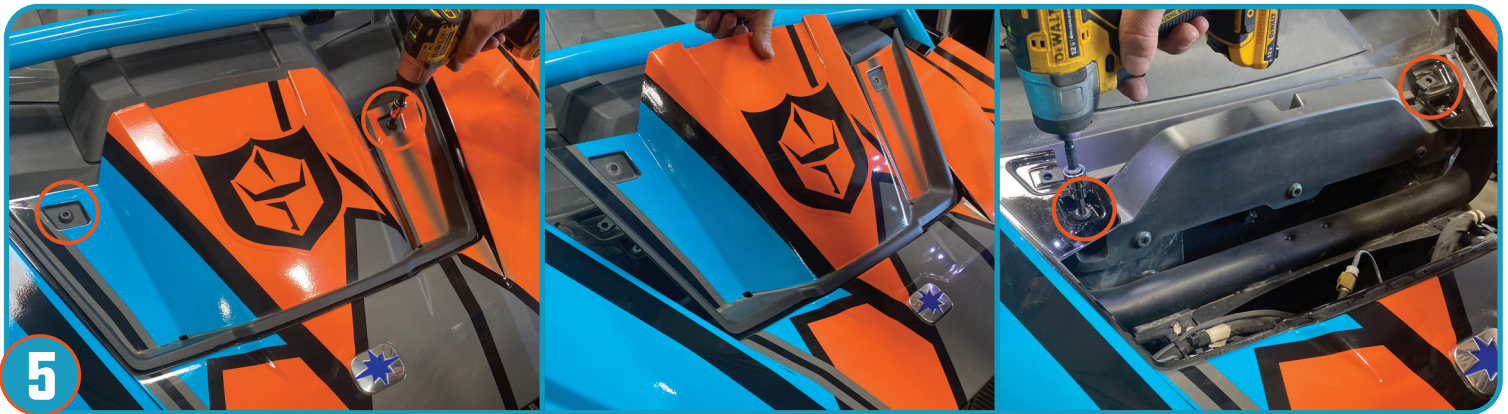
5 REMOVE THE HOOD PLASTICS (2-BOLTS). REMOVE TWO BOLTS LOCATED UNDER HOOD, AS SHOWN.
