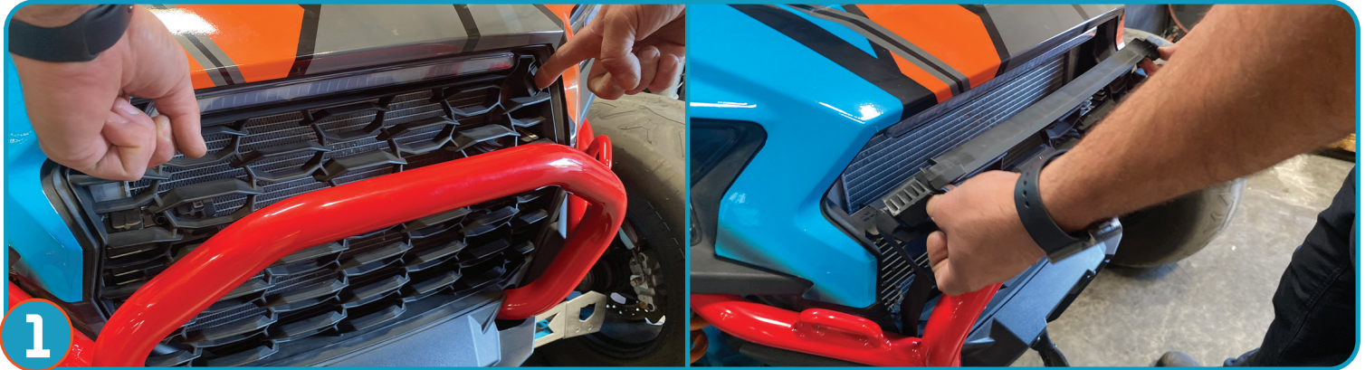
1 REMOVE STOCK GRILLE BY DEPRESSING THE TWO CLIPS ON EITHER SIDE OF GRILLE AS SHOWN.
