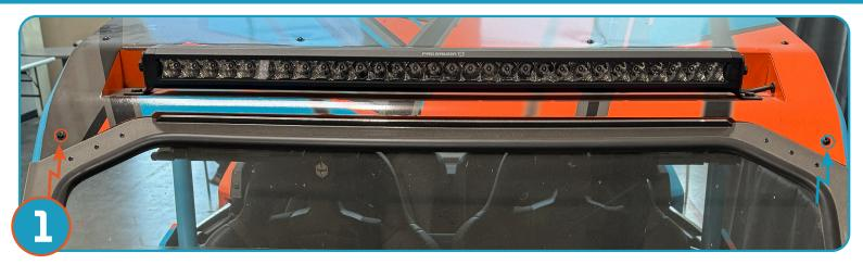
If roof already installed, remove top two roof screws and place windshield on the vehicle, sliding top of windshield under roof and lining up bolt holes. Use provided hardware.
