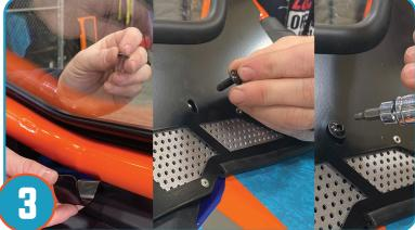
Using the provided (2) brackets/bolts, secure the lower windshield tightening the bracket, threading bolt from outer windshield to cage. One bracket per side of windhshield.
