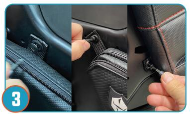
Line up remaining 3 mounting points, utilizing the same bolts removed in step-1 and tighten. Repeat for opposite door.
