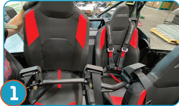
1 Remove stock seat from vehicle by reaching behind seat and pulling on the release handle (Red)
