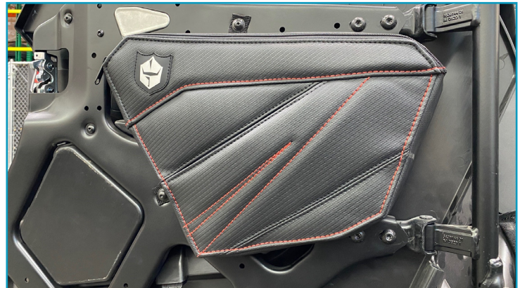
Starting with mounting bolt inside the door bag pocket. Line up bolt with mounting point (closest to hinge) on door and tighten.
