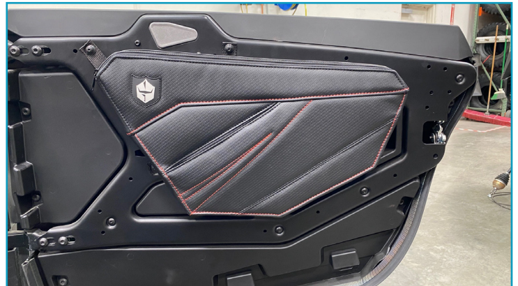
Starting with mounting bolt inside the door bag pocket. Line up bolt with mounting point (closest to latch) on door and tighten.
