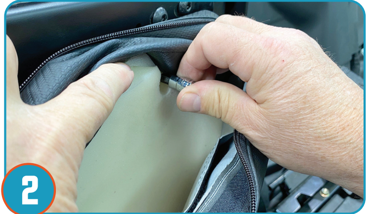
Starting with mounting bolt inside the door bag pocket. Line up bolt with mounting point (closest to hinge) on door and tighten.
