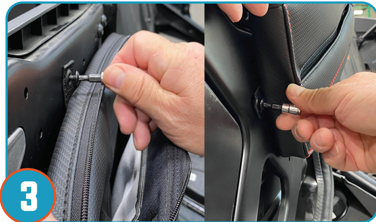
Line up remaining 2 mounting points, utilizing the same bolts removed in step-1 and tighten. Repeat for opposite door.
