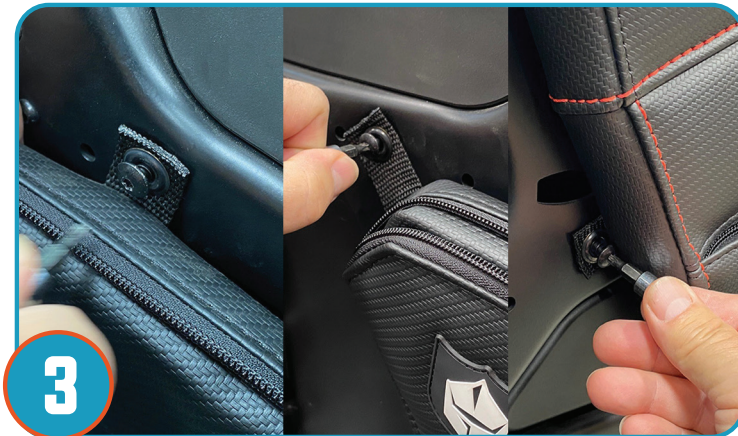
Line up remaining 3 mounting points, utilizing the same bolts removed in step-1 and tighten. Repeat for opposite door.
