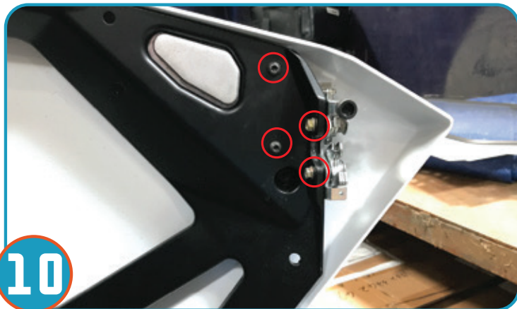
10 Remove 4 bolts holding the OEM Paddle latch and slam latch on the stock door. Repeat for opposite side.
