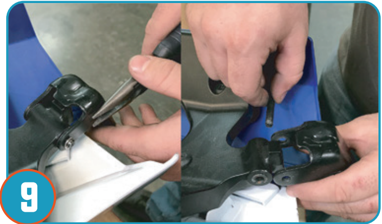
9 Stock hinges will be used for your Pro Armor door. Remove hinge by carefully removing the clip and sliding the pin from the hinge. Remove hinge from stock door. Remove bushings from door. Repeat for opposite door.
