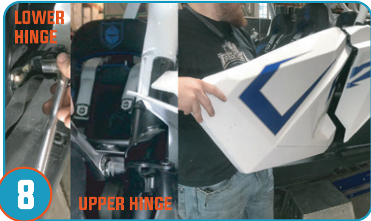
8 Remove stock door by removing 4 bolts per door and remove lower & upper hinge to remove door from vehicle. Repeat for opposite door.
